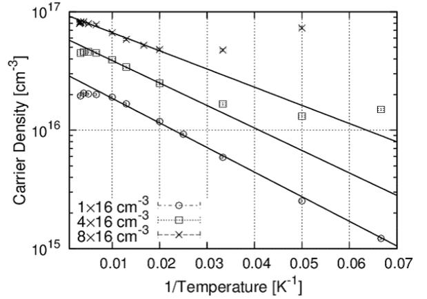
Figure 2. Carrier densities as a function of temperature.
