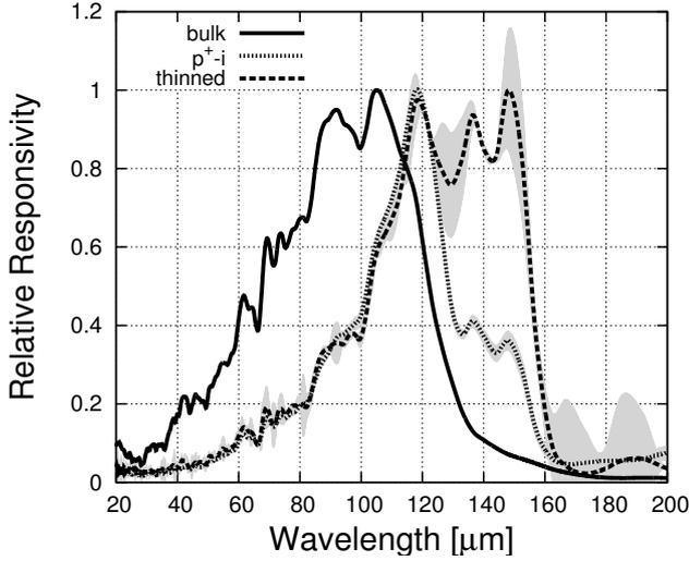
Figure 1. Spectral response curves for the three devices. The vertical axis shows the relative responsivity where the peak is normalized to a unity for each device. The hatched regions represent  $1\sigma$  errors.
