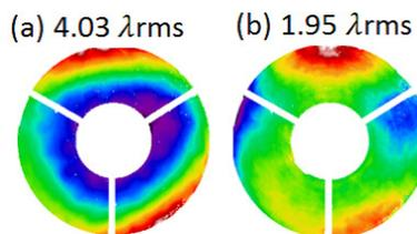
Figure 5. The WFE maps derived with the deformed ACF (a) before correction and (b) after correction.
