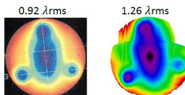
Figure 4. Largely deformed  $\phi$ 300-mm ACF. (Left) The SFE of the ACF. (Right) The SFE derived by our new method.
